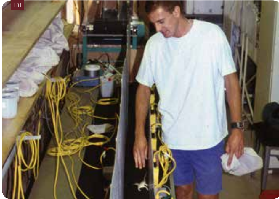
Photocell-lined racetrack connected to a computer used to measure maximal running speeds of lizards. Lizards are chased by hand which simulates a predator
